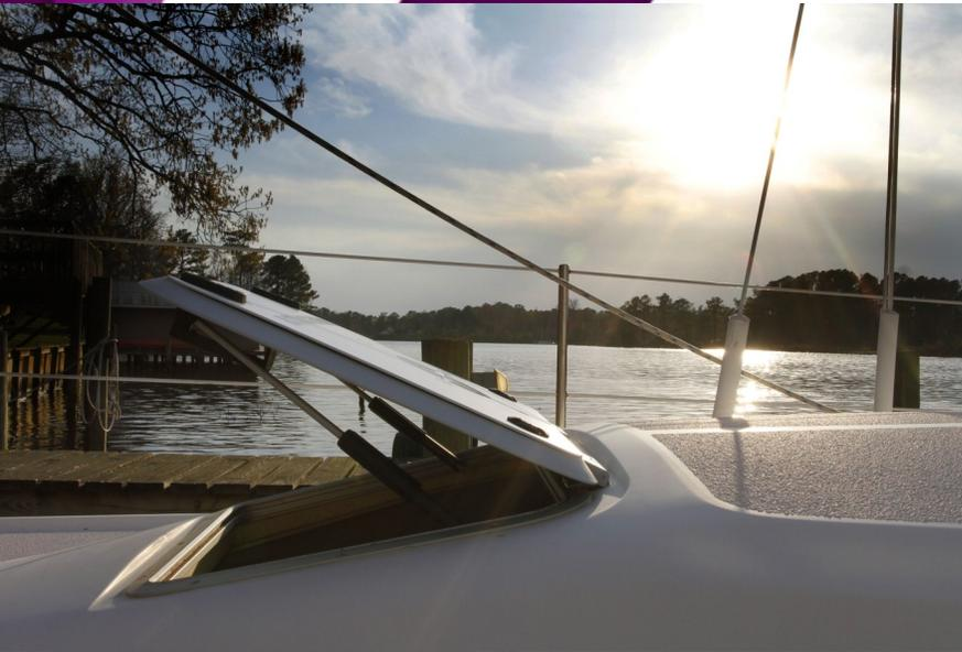
Outland Hatch Covers, based in Jacksonville, NC, owned by twin brothers Steve and James Outland, has found a successful use of Vycom's Celtec material for fabricating their new boat hatch covers, which provides UV protection for the acrylic lens of deck hatches.
